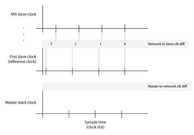
In phase 2, the algorithm shifts the sample time of the master stack running on the target computer to align with the first slave node clock. In that process, the EtherCAT Init block output value <code>MasterToNetworkClkDiff</code> decreases to near zero.
