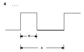
For a base frequency b, this algorithm results in a rectangular output signal of frequency b/n and duty cycle m/n. Because m and n must be integers, it is not possible to provide a continuous range of output frequencies and duty cycles with perfect exactness.
