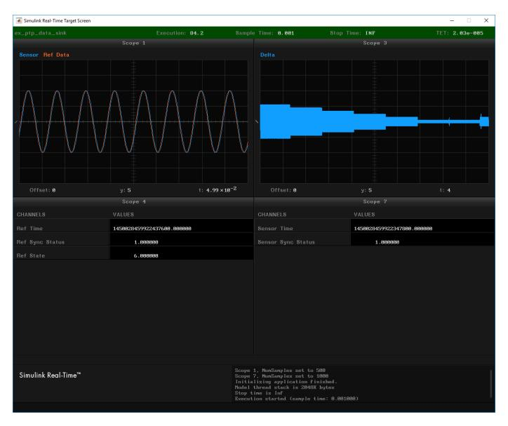
With the IEEE 1588 Sync Execution block, you can make measurements across multiple target computers at a synchronized time step. However, the kernel interrupt clock controller can shorten some time steps up to 10% of the fundamental sample time, resulting in a CPU overload.
