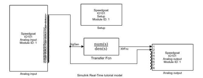
You cannot run this model unless the required I/O board is installed in your target computer. However, you can substitute driver blocks for another I/O board that is installed in the target computer.
