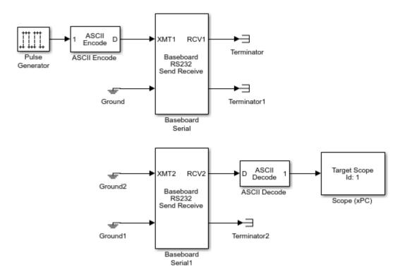
14 Double-click a Baseboard RS232 Send Receive block. To configure the ports on the target computer for this board, enter values.
