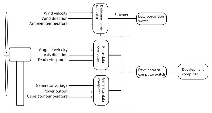
To record the data and timestamps, you connect the sensors to a set of data acquisition target computers. You interconnect the data acquisition computers through an Ethernet network and a switch that supports the PTP protocol (a PTP transparent clock or boundary clock). To access the data and timestamps, you connect the target computers to a development computer through another Ethernet network and switch. On the development computer, you run MATLAB to do the data analysis, including:
