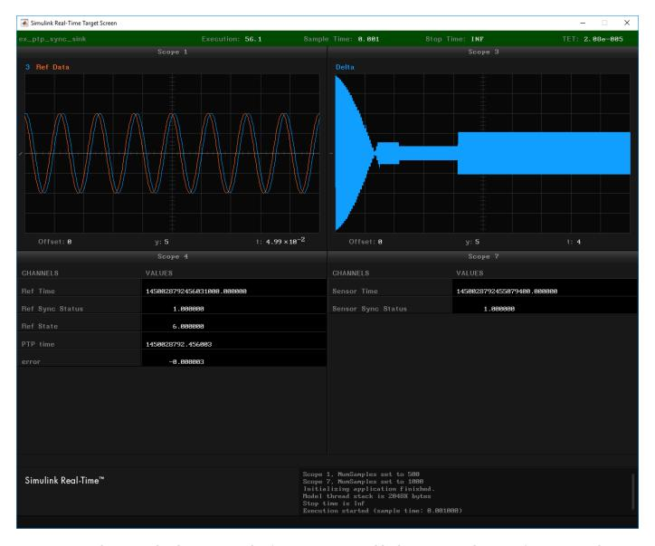
For this example, the sensor and reference Sine Wave blocks are set to the same frequency and amplitude, but start at arbitrary times. The difference in start time causes a phase difference between the sine waves. The phase difference appears on the <code>Delta</code> scope as a waveform that settles to a constant amplitude.
